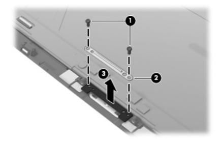
Reverse this procedure to install the home button board and bracket.
